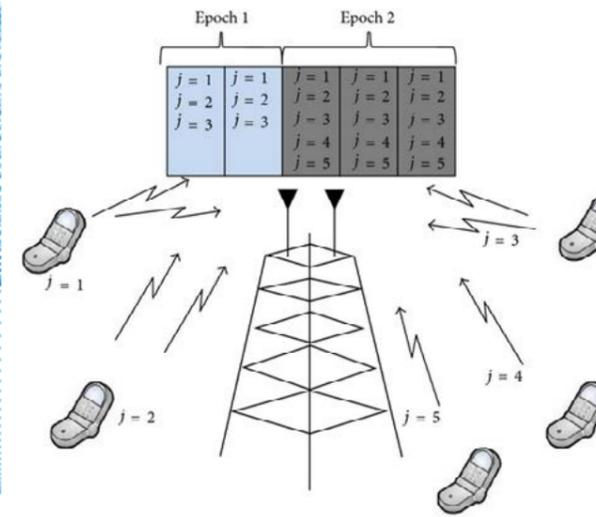
Fig. 1 Random-access network assisted by retransmission diversity and multipacket reception.
