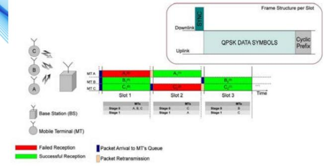
Fig. 2 PC ARQ prefix-assisted DS-SS-CDMA Reception scheme example and frame structure per slot.
