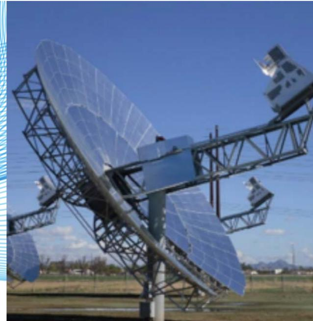
Fig. 1 A Biostirling parabolic concentrator with its Stirling engine at its focus.
