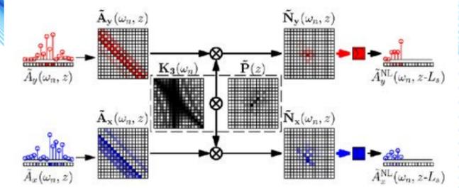
Fig. 2 Parallel implementation of the dual-polarization VSNE algorithm.
