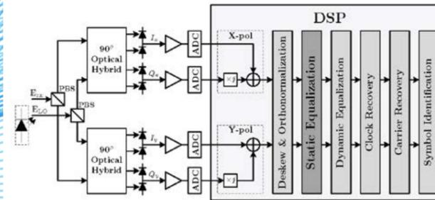
Fig. 1 Physical structure and general DSP subsystems of a polarization-diversity digital coherent optical receiver.
