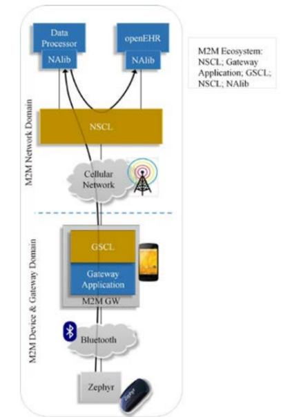
Fig. 2 Overview of deployed mobile IoT application with service composition using ETSI M2M for interoperability.
