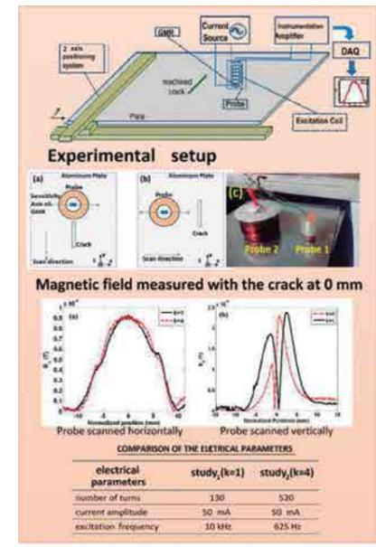
Fig. 2 Detection of cracks by eddy current testing based on dilation invariance principle.
