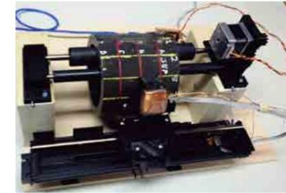
Fig. 1 Eddy currents based system to characterize HP Steel.
