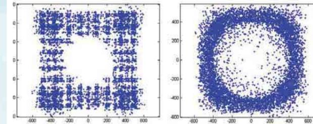
Fig. 1 IQ transition Diagram of bandwidth Limited OQPSK signal with and without the use of RMM technique, obtained with the SDR implementation prototype.
