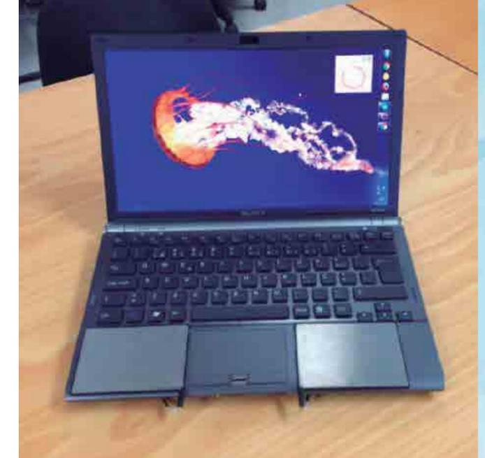
Fig. 2 VitalityType prototype for near-continuous ECG monitoring while using the computer.
