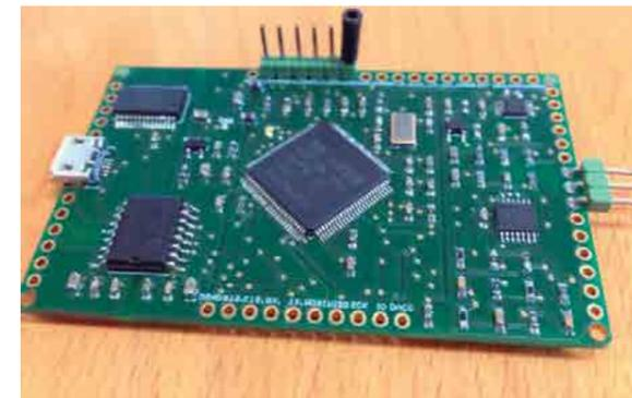
Fig. 1 Instrumentation for pervasive Electrocardiography (ECG).
