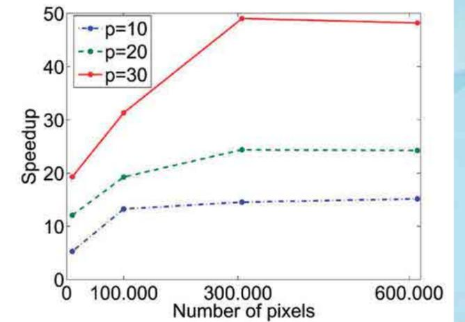
Fig. 2 Speedup of PSISAL method on GPU as a function of the number of endmembers and of the image size.
