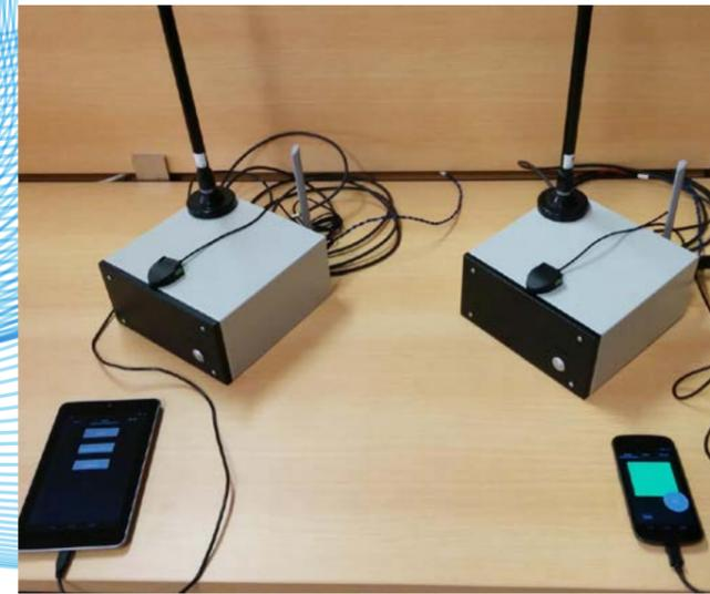
**Fig. 1** ITS G5 stations (IT2S) with external antennas (GPS and 5.9 GHz) and Android devices.
