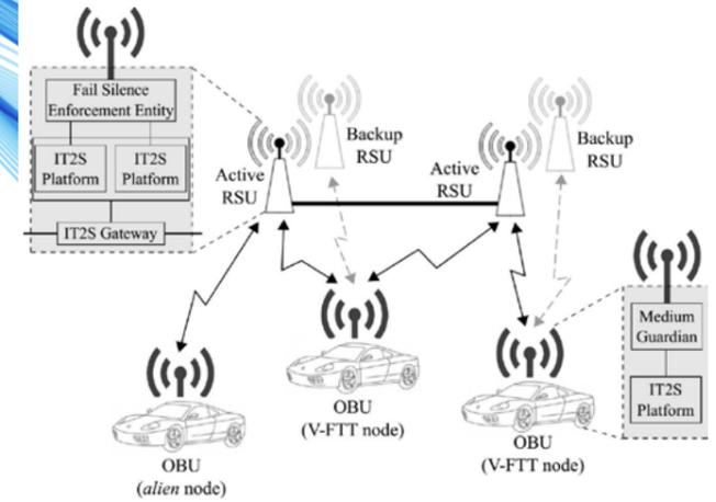
**Fig. 2** Dependable vehicular network architecture proposed in the scope of ICSI project.
