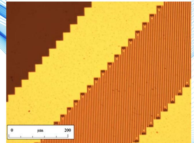
**Fig. 2** Detail of interdigital transducer of uncoated die.
