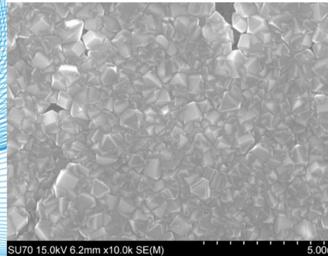
**Fig. 1** Scanning electron microscope image of diamond film deposited on lithium niobate.
