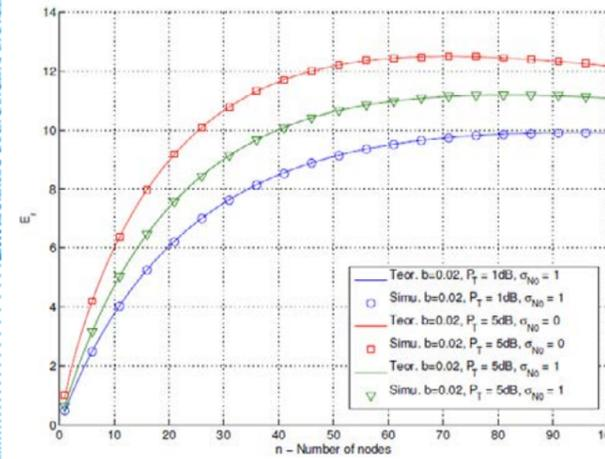
Fig. 1 M2O physical-layer model: average number of packets successfully received ( $E_r$ ) when  $n$  nodes simultaneously transmit.
