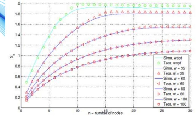
Fig. 2 Throughput evaluation of multiple parameterizations of the proposed M2O MAC protocol for different number of competing nodes.
