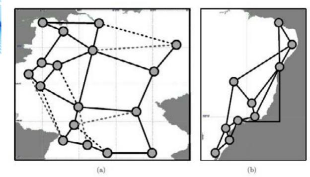
Fig. 2 Topologies obtained using the Integer linear programming model and the genetic algorithm for the node location of (a) German network and (b) Brazilian RNP network.
