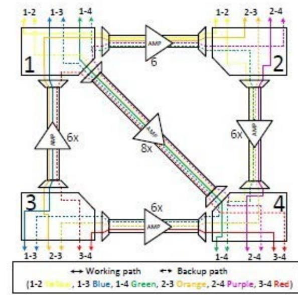
Fig. 1 Dimensioned network corresponding to a feasible solution for the survivable topological design problem.
