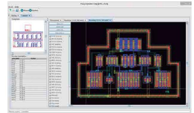
Fig. 2 AIDA-L Analog IC Layout Generation and Graphical User Interface.
