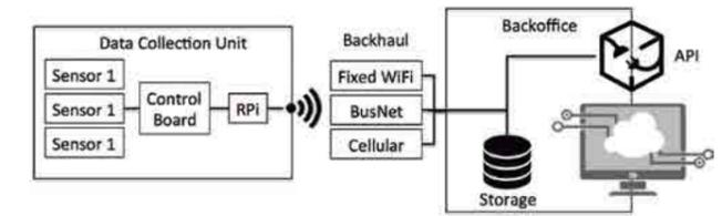
Fig. 2 SenseBusNet Architecture.
