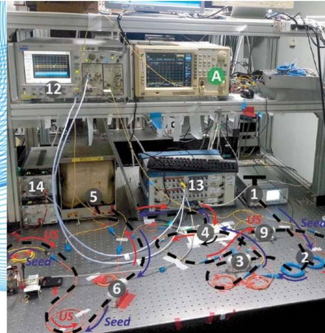
**Fig. 1** Laboratory system assembly for remotely seeded reflective PON, based on upstream (US) signal generation by means of RSOA.
