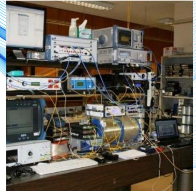
**Fig. 2** Laboratory UDWDM and DWDM demo setup, with fiber and free space optics infrastructures
