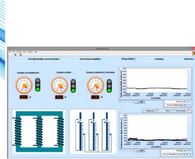
Fig. 2 User interface of the application developed showing the condition of the power transformer
