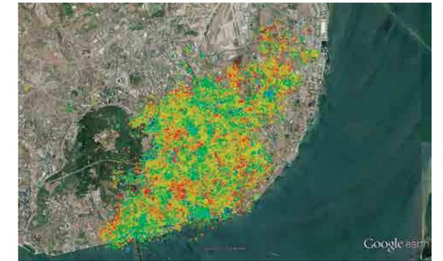
Fig. 2 Base-station signal level footprint for central Lisbon after geolocating network recordings (traces).
