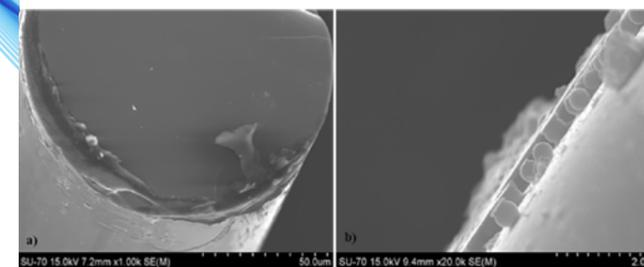
**Fig. 2** SEM images of (a) transversal and (b) longitudinal cut of silica-coated TFBG.
