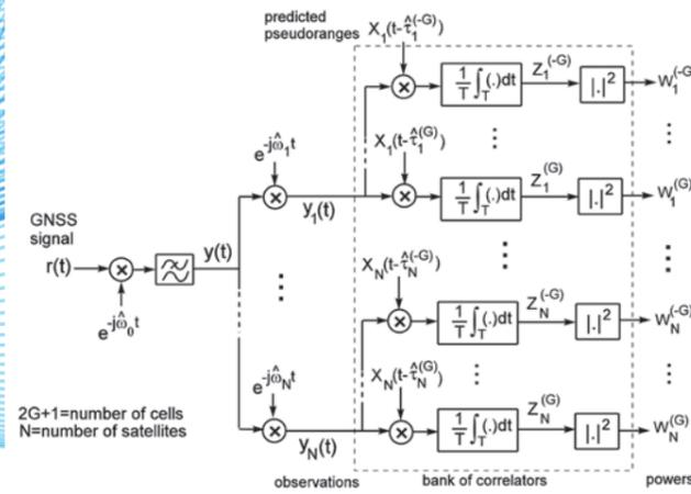
Fig. 1 Pre-processing part of the proposed low-complexity VDLL architecture
