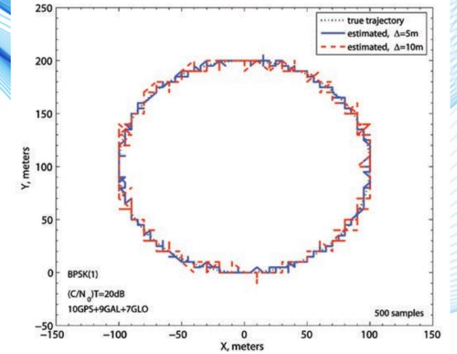
Fig. 2 Circular trajectory estimation with 500 samples, different cell sizes, and BPSK(1) modulation
