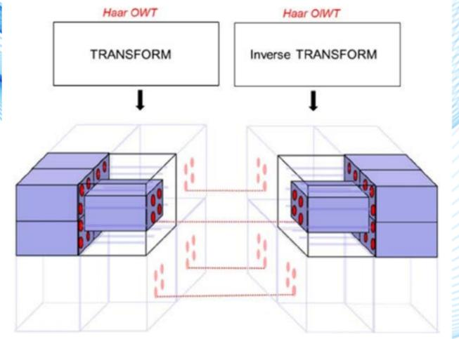
**Fig. 2** Integrated passive scheme for Optical Wavelet Transform and Inverse Wavelet transform (WT-IWT); passive compression is accomplished by spatial selection of LL coefficients, delivered through reported connections.
