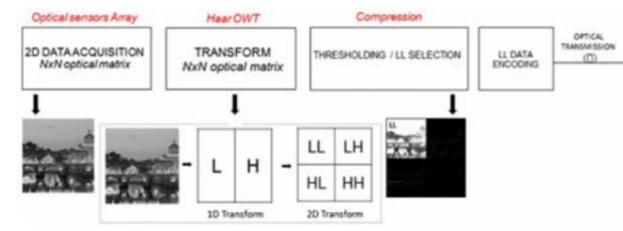
**Fig. 1** System building blocks for Haar optical wavelet transform (OWT) based on all-optical processing and compression. 2D transform process schematic describes low-pass (L) and high-pass (H) filtering until sub-band decomposition.
