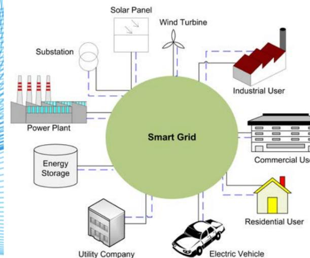
**Fig. 1** Smart Grid establishes two-way power and information flows between the grid and the end-consumers, enabling distributed generation and storage.
