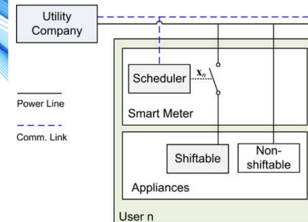
**Fig. 2** The scheduling algorithms defer only the user's shiftable appliances (e.g., Electric Vehicle changing), without interfering her non-shiftable ones (e.g., cooking appliances, ITlights, etc.)
