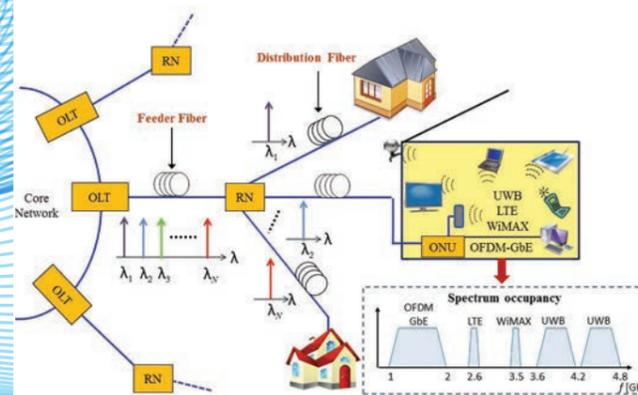
Fig. 1 Schematic diagram of the FIVER network proposed for the quintuple-play service provisioning.
