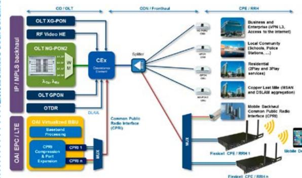
Fig. 1 Deployment scenario of the Flexicell project in the scope of Radio Access Network converged with a Passive Optical Network infrastructure.
