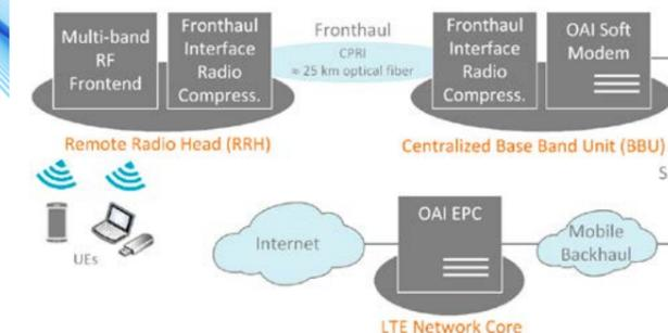
Fig. 2 Architecture of the Flexicell lab demonstrator, including the interoperability and connectivity with user terminals.
