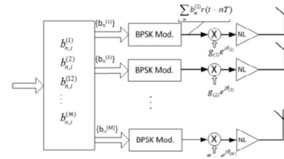
Fig. 1 Transmitter structure.
