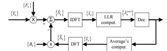
Fig. 2 Receiver structure with detail of the decision block in the uncoded (A) and coded (B) cases.
