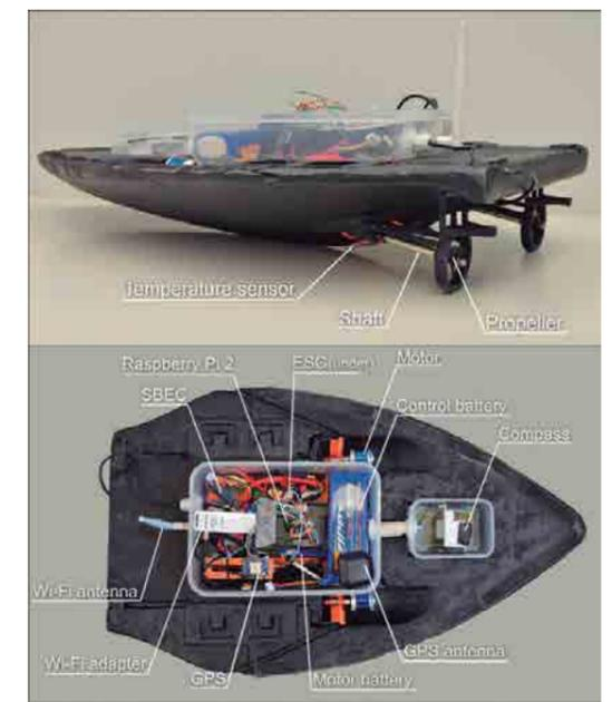
Fig. 2 Aquatic drone hardware developed.
