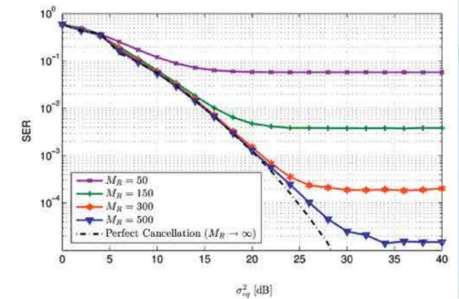
Fig. 2 End-to-end symbol error rate in the two-way relay channel applying physical layer network coding, using a massive mimo relay (for a varying number of antennas) operating in full-duplex.
