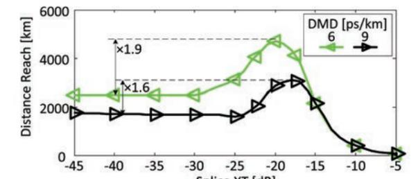
Fig. 2 Distance reach as a function of splice XT.
