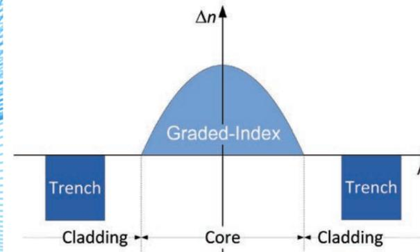
Fig. 1 Refractive-index profile composed by a graded-index core and a cladding trench.
