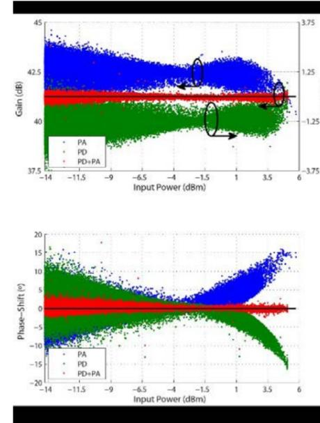
**Fig. 1** Final gain and phase-shift characteristics of the original PA, of the linearized PA and of the complete predistorter.
