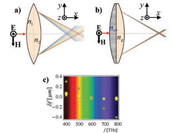
**Fig. 2** (a) Illustration of the chromatic aberration of a conventional glass lens. (b) Biconvex optical metamaterial lens that corrects the chromatic aberration for all the colors of light. (c) Yellow stars/circles: focal curve for the compensated metamaterial lens. Diamond symbols: focal curve for a conventional single-material lens.
