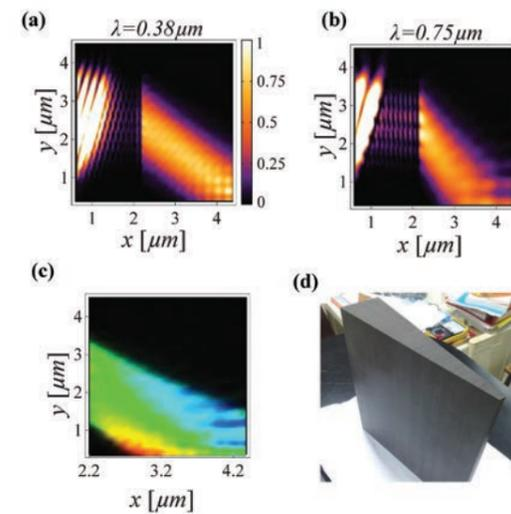
**Fig. 1** A nonlocal metamaterial prism refracts long wavelengths more than short wavelengths (panels a-b), producing a reversed rainbow (panel c). Panel (d) shows a prototype of the metamaterial prism used to experimentally demonstrate this effect at microwaves.
