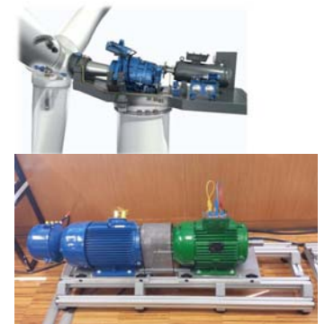
Real-time diagnostic system for wind generator
