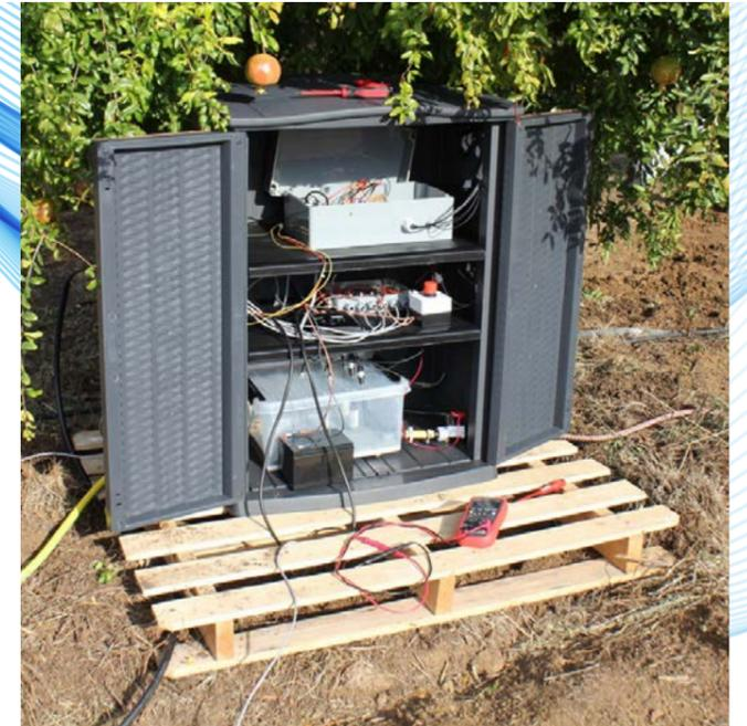
Fig. 2 Initial prototype of the water sampling unit and general connectivity.
