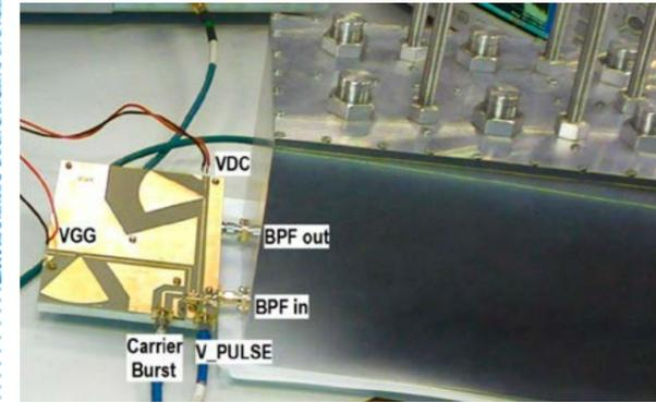
Fig. 1 RF transmitter with cavity filter.
