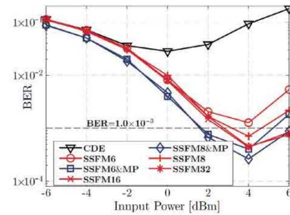
**Fig. 1** BER improvement as a function of input power for DBP-SSFM (red curves) and DBP-SSFM aided with Memory Polynomial (blue curves) for a total link length of 800 Km.
