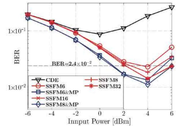
**Fig. 2** BER improvement as a function of input power for DBP-SSFM (red curves) and DBP-SSFM aided with Memory Polynomial (blue curves) for a total link length of 1600 Km.
