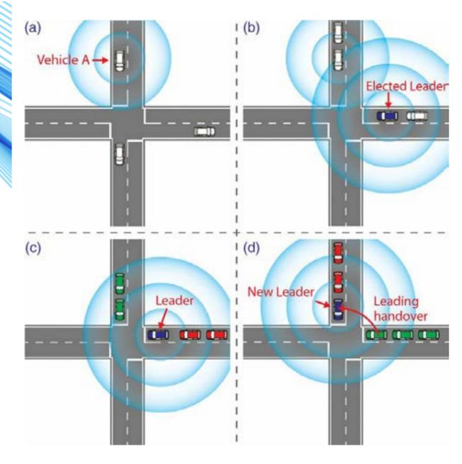
Fig. 2 Virtual traffic lights operation.
