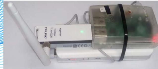
Fig. 1 Prototype developed with RPi.
